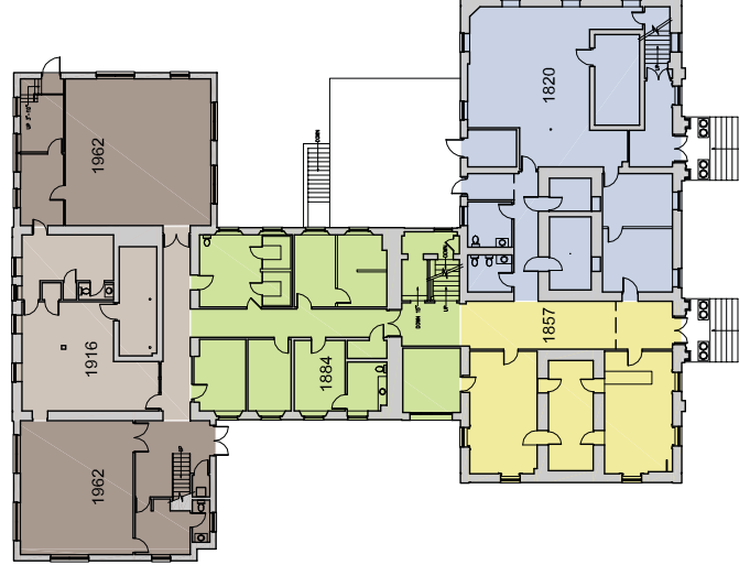
Stages of Courthouse construction
